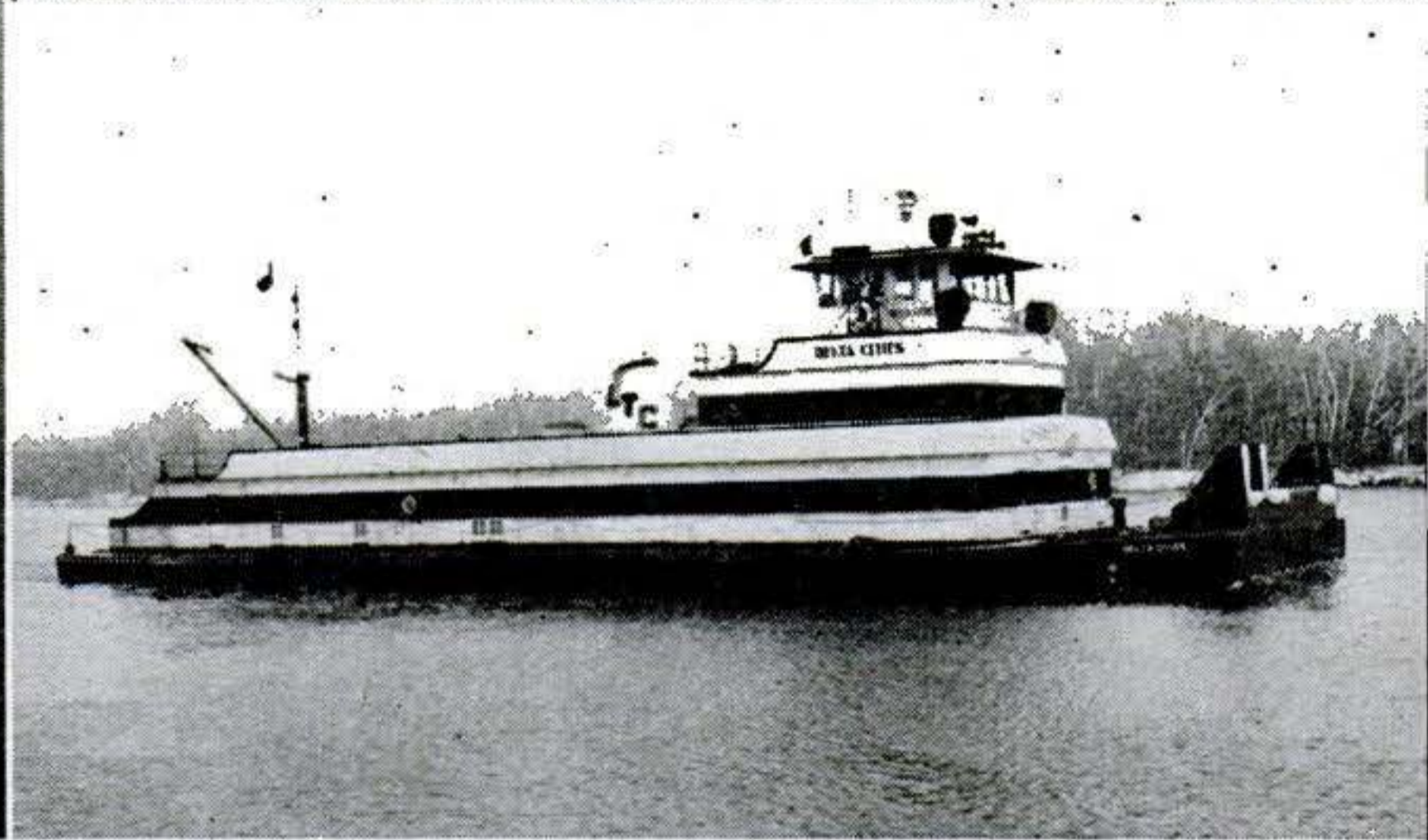
TWO NEW TWIN-SCREW DIESEL TUGS. Top the handsome Lady Linda . Bottom: the 3,200-hp. Delta Cities (PSM, Jan. '52, p. 108).
